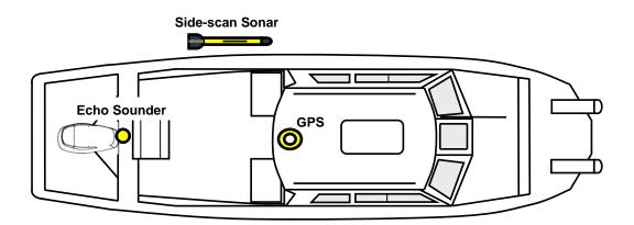
Figure 1. Equipment layout for the survey vessel.
